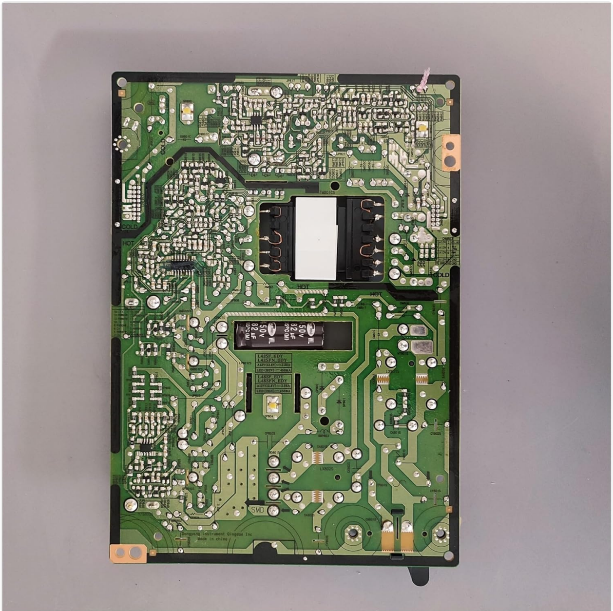
Figure 2: Bottom view of the power board. This perspective shows the intricate circuit traces and solder points that connect the components on the top side, essential for power distribution and signal integrity.
