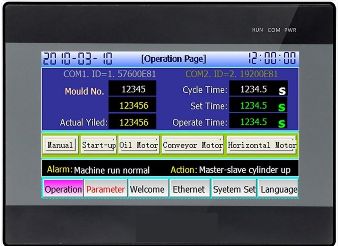
Figure 2: Front view of the HMI PLC unit showing an example "Operation Page" with English labels. This interface allows users to input data (e.g., Mould No., Cycle Time), view real-time status (e.g., Actual Yield, Alarm messages), and control operations via touch buttons (e.g., Manual, Start-up Oil Motor).
