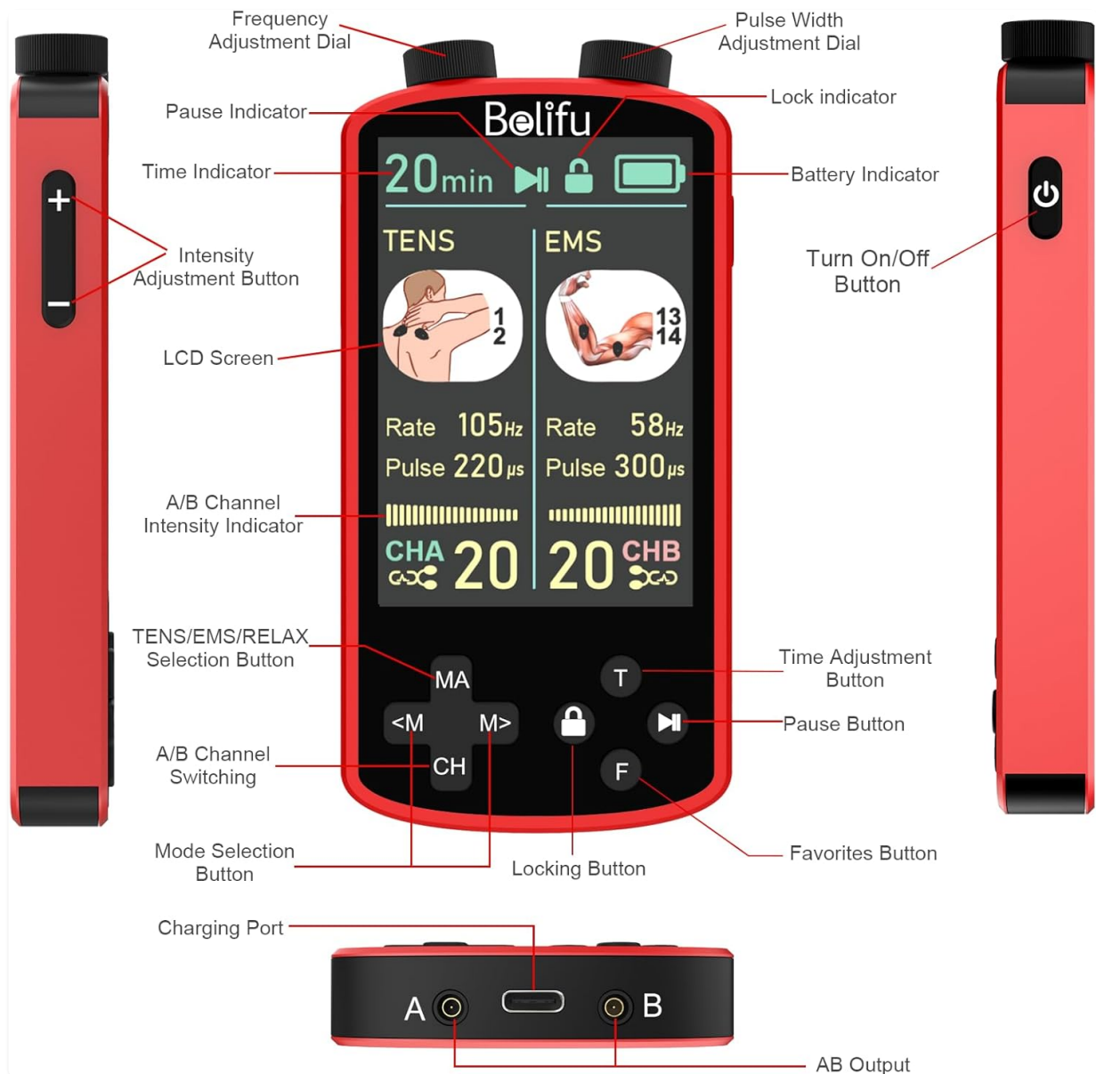
Image 6.1: Labeled diagram of the Belifu TENS EMS Unit's controls and display.
