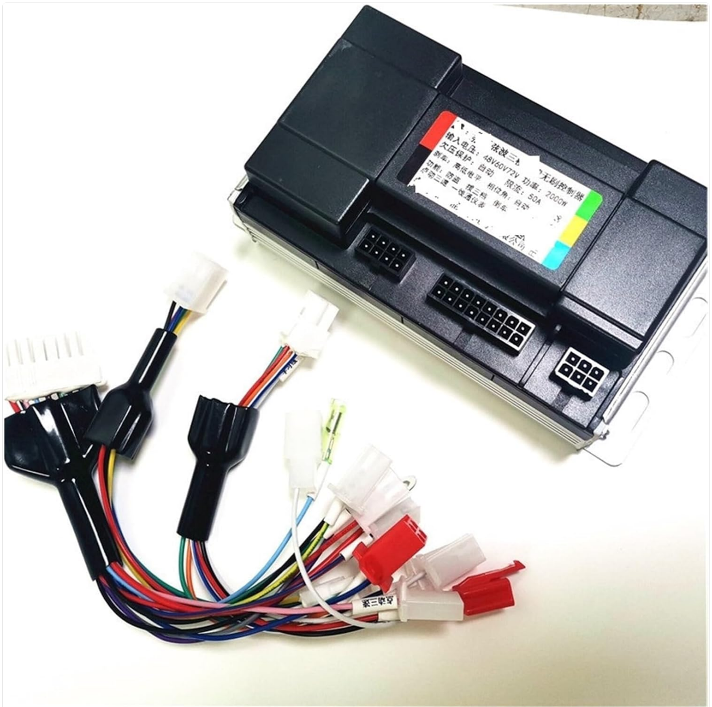
Figure 3.3: The JIANGFAN controller shown alongside its wiring harness. This view provides a perspective of the controller's size relative to its connections and illustrates how the harness integrates with the main unit.
