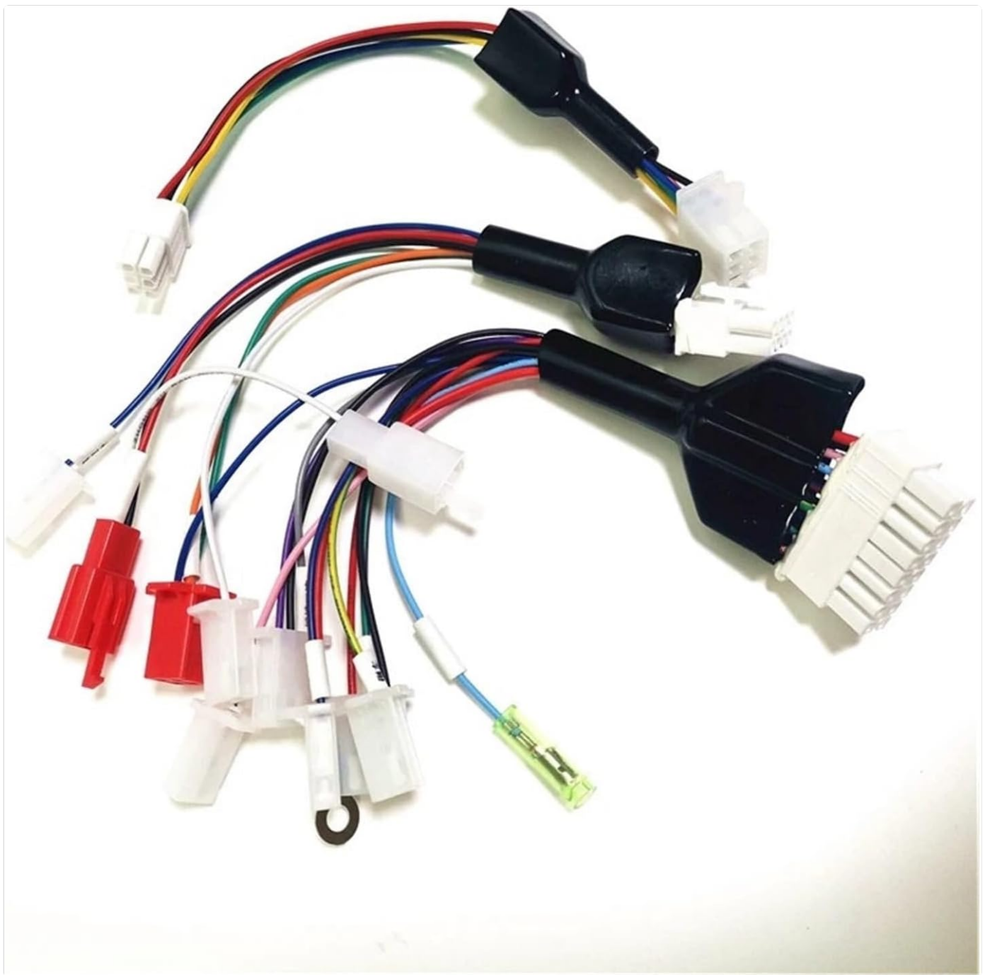
Figure 3.2: The complete wiring harness for the controller. This image displays the various color-coded wires and connectors, essential for connecting the controller to the motor, battery, throttle, and other vehicle components.
