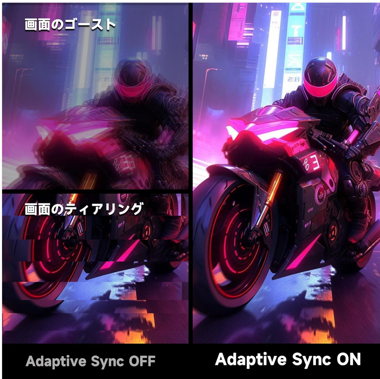
Image 4.2: Visual comparison demonstrating the effect of Adaptive Sync being OFF (showing ghosting and tearing) versus ON (smooth image).
