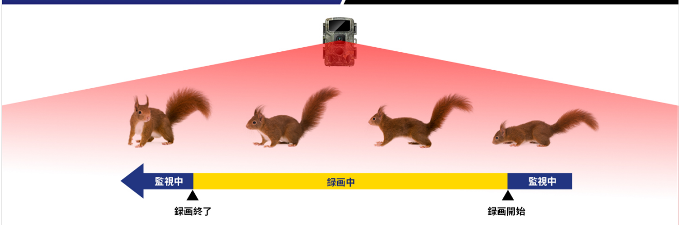
Image: PIR motion detection automatically triggers recording when movement is detected.
