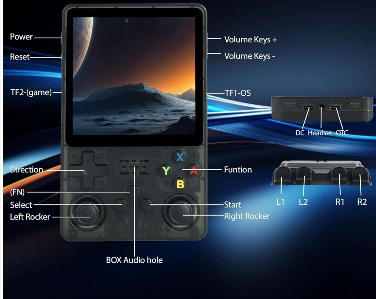
Figure 2: Detailed view of the console's optimized key layout.
