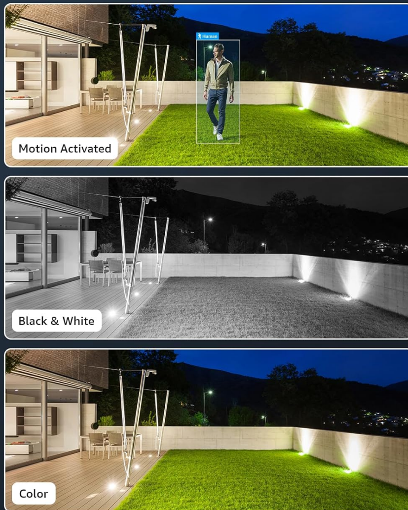
Image: A comparison of three night vision modes: 'Motion Activated' (showing a human detected in color), 'Black & White' (standard infrared night vision), and 'Color' (full-color night vision in low light).
