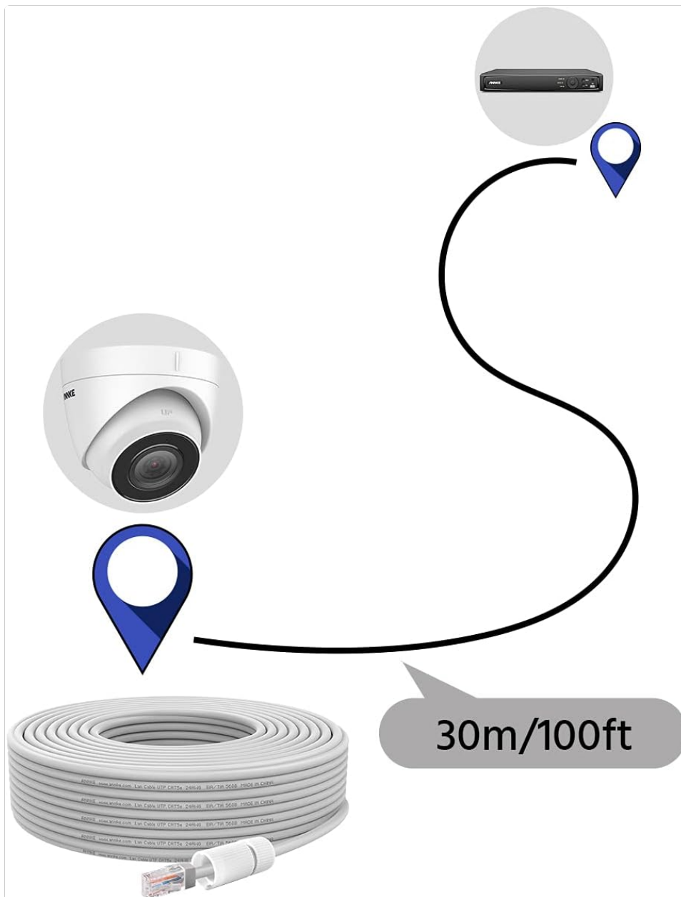
Image: A diagram illustrating the simple connection path of a PoE camera to the NVR using a single Ethernet cable, indicating support for cables up to 100ft (30m).
