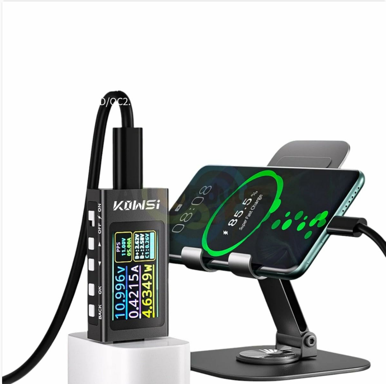
Figure 4.1: KWS-X1 Type C Voltage and Current Detection Monitor in operation, showing its compact design and clear IPS display. The display shows real-time voltage (10.996V), current (0.4215A), and power (4.6349W) readings, along with battery percentage (85.5%) and charging status.
