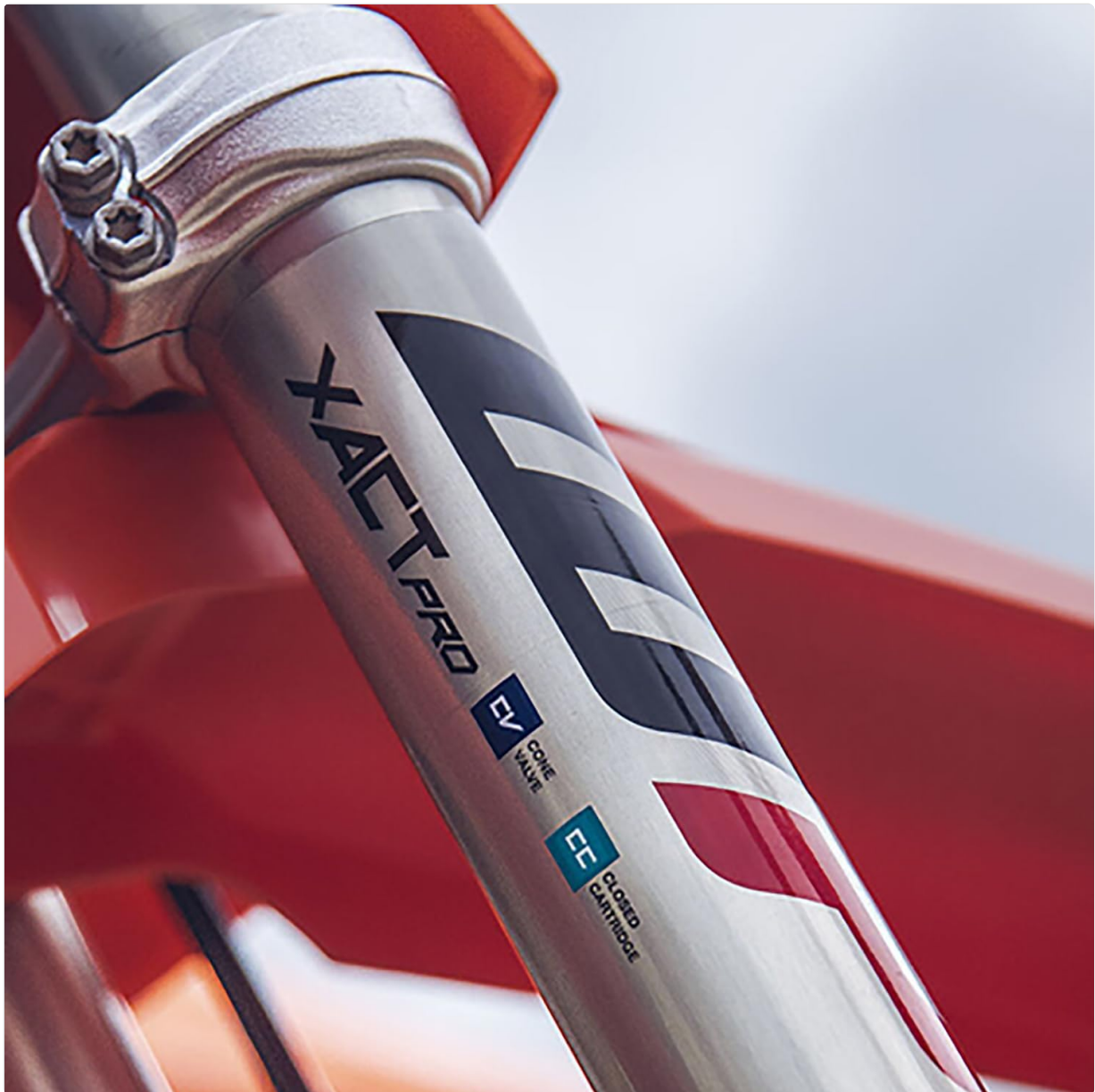
Image 2.1: XACT PRO Technology Details. This close-up image highlights the 'XACT PRO' branding along with 'Cone Valve' and 'Closed Cartridge' indicators on the fork leg, signifying advanced internal technology.
