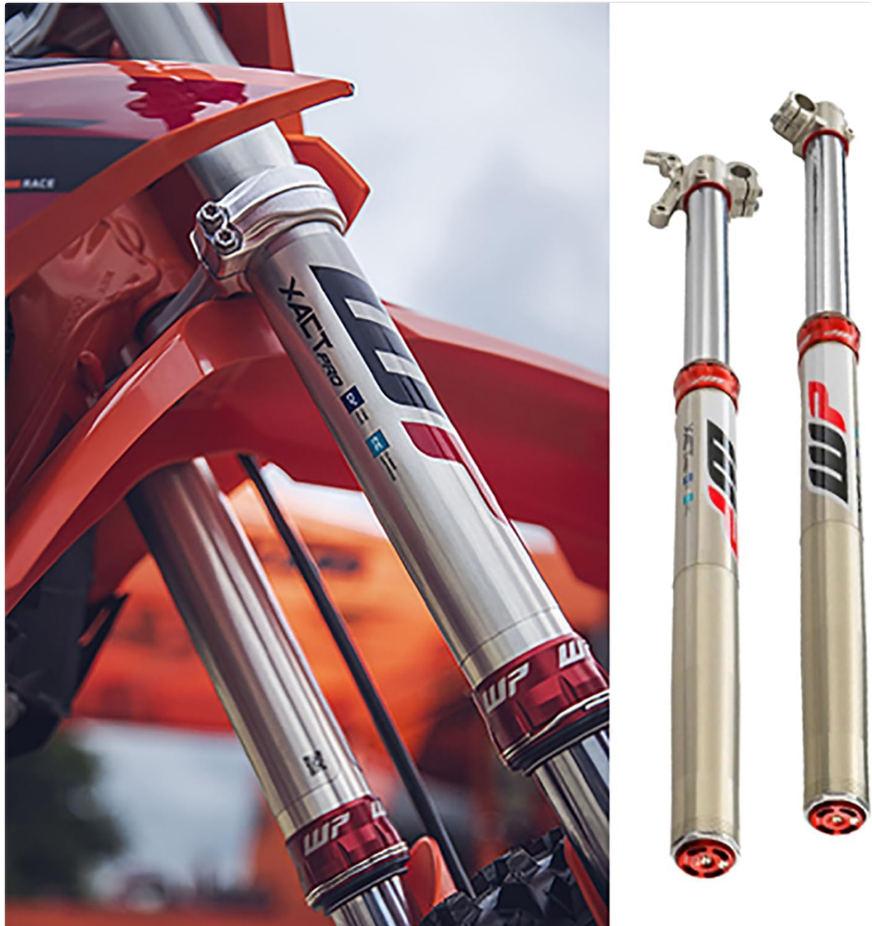
Image 4.1: Forks Installed on a Dirt Bike. This image shows the WP XACT PRO forks mounted on a motocross bike, demonstrating their appearance in an operational context. A smaller inset displays the forks individually.
