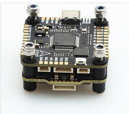
Image 1: Assembled F722 Flight Controller and BLS-60A 4in1 ESC stack.
