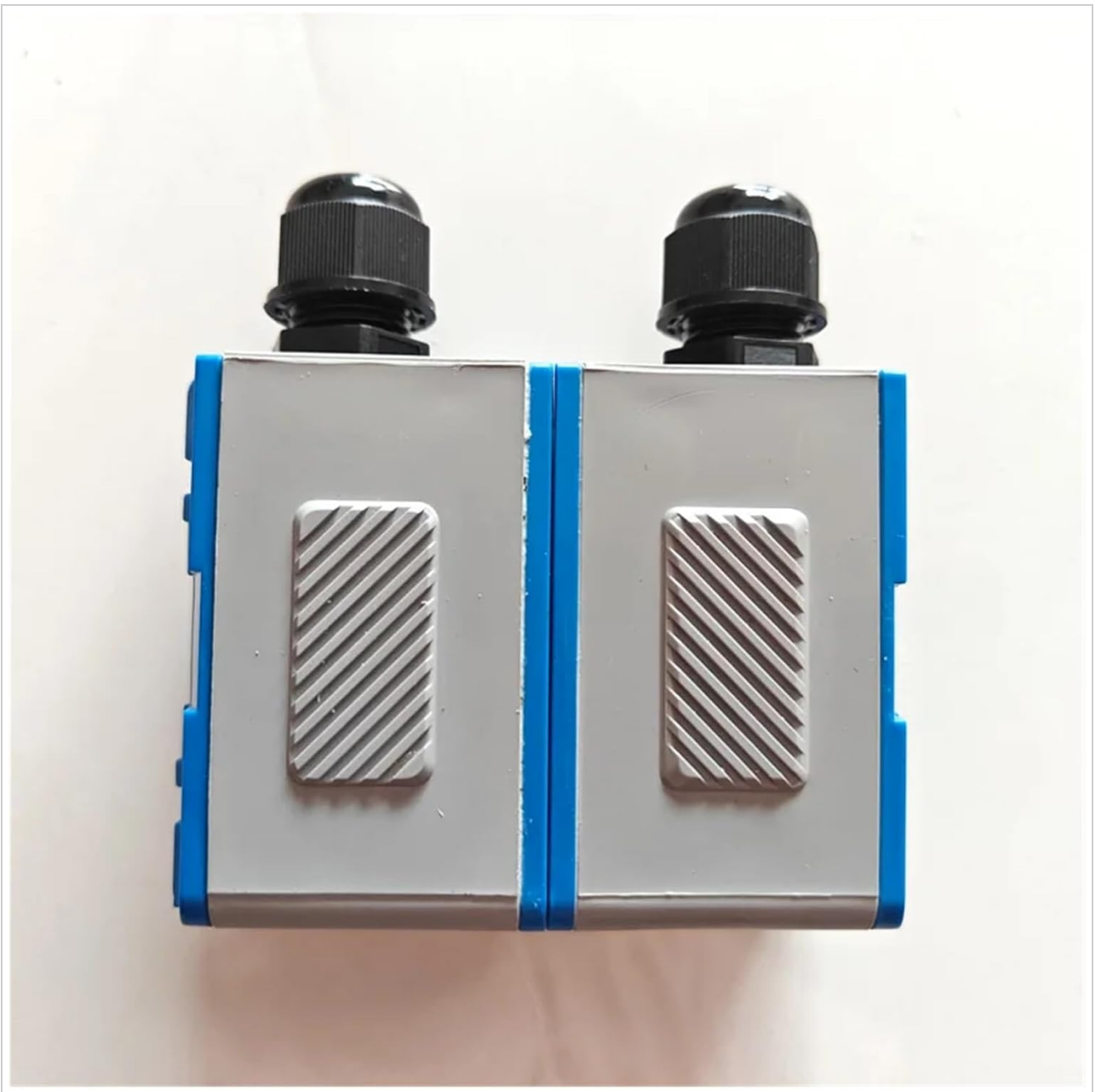
Figure 5.3: Close-up view of the clamp-on ultrasonic transducers, which attach to the exterior of the pipe.
