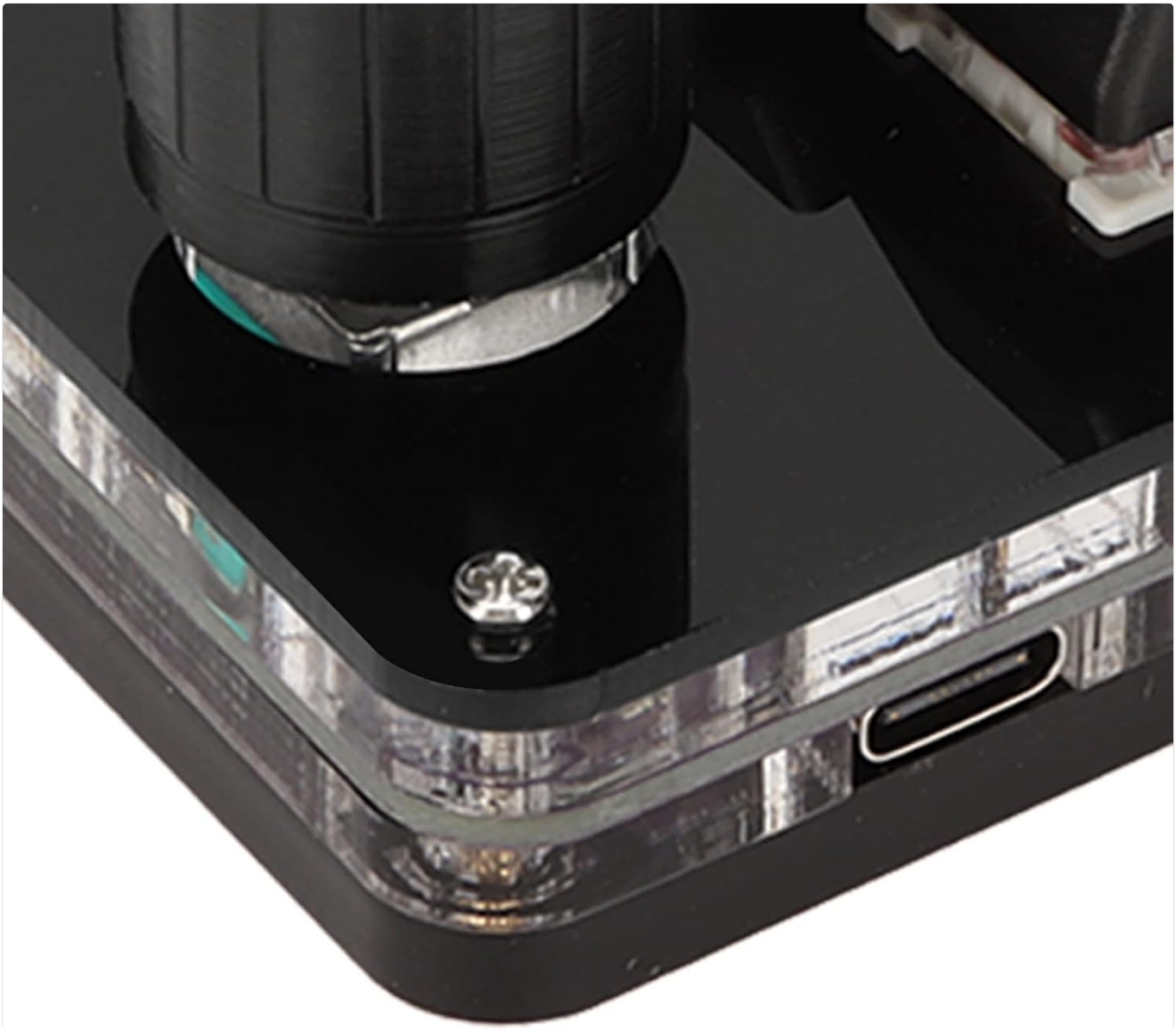
Image 2.2: A detailed view of the USB Type-C port on the side of the macro keyboard, where the data and power cable connects.
