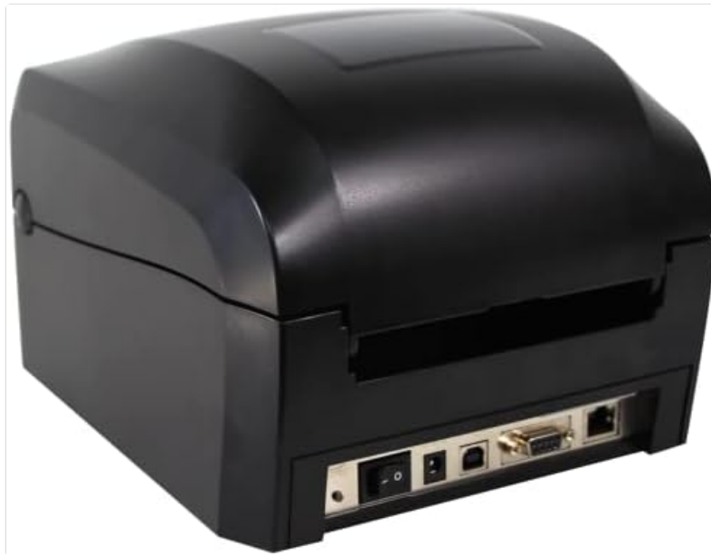
Image: Rear view of the Godex GE300 printer, highlighting the USB, Ethernet, and Serial connectivity ports for easy integration with various systems.
