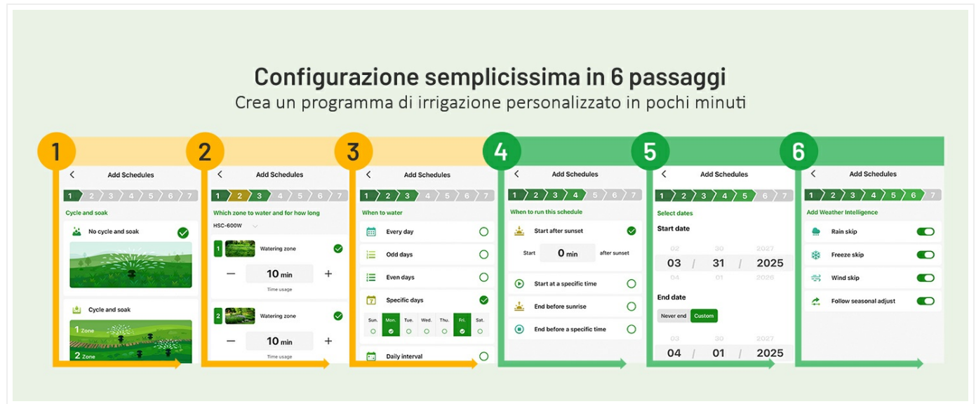
Figure 5: The 6-step process for creating a personalized irrigation schedule using the HiOazo app.
