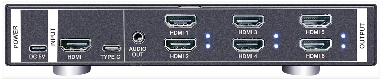
Figure 4.1: Front Panel Layout
