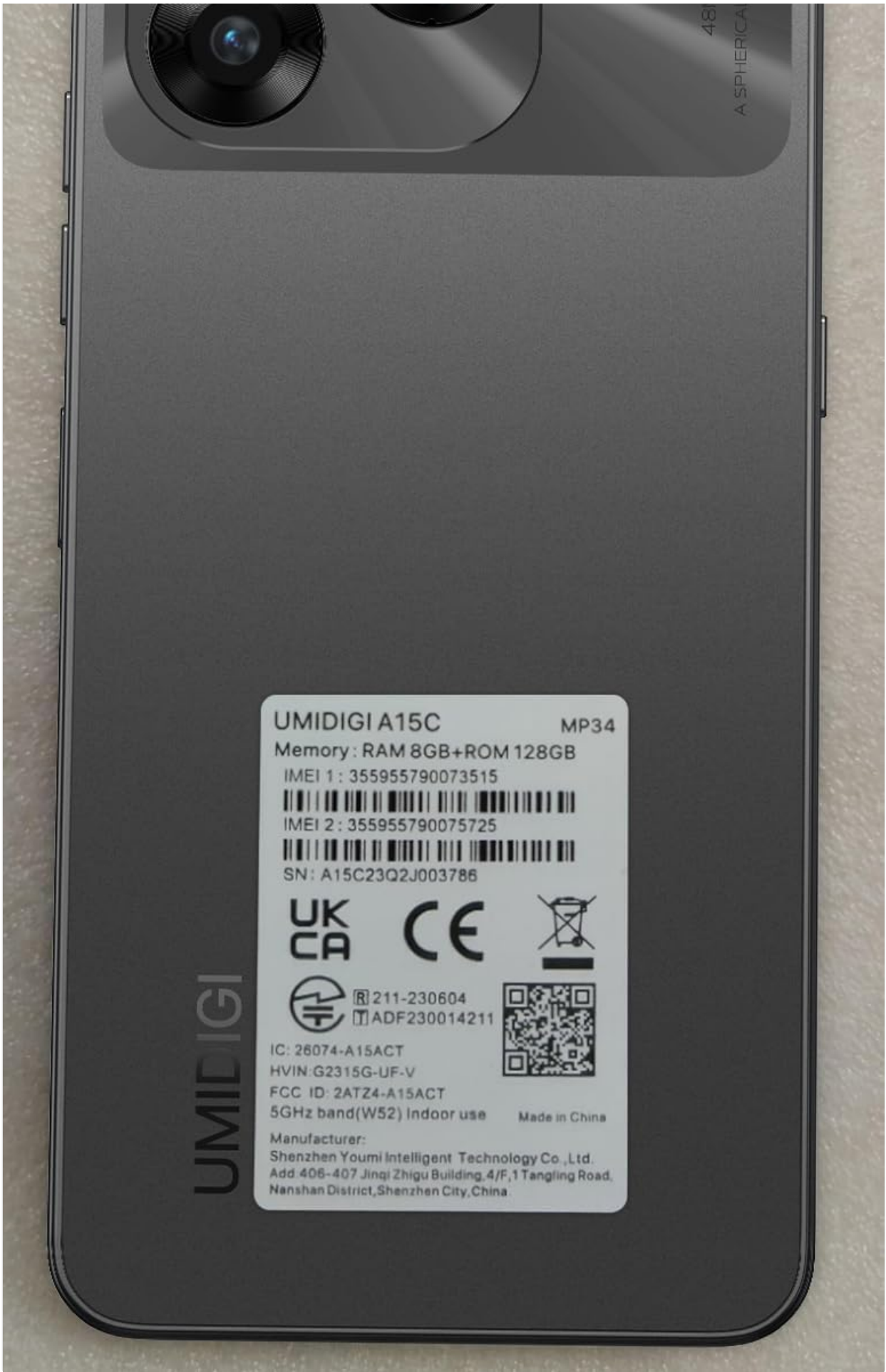
Figure 9.1: Rear view of the UMIDIGI A15C with its product information label, indicating model, memory, and regulatory compliance details.
