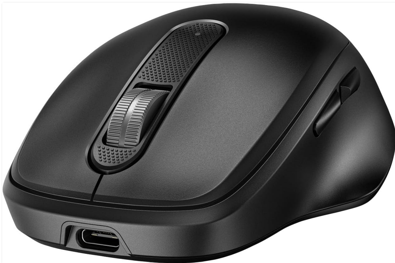
Figure 1: Front view of the HP 515 Wireless Mouse, showing the left and right click buttons, scroll wheel, and USB-C charging port at the front.
