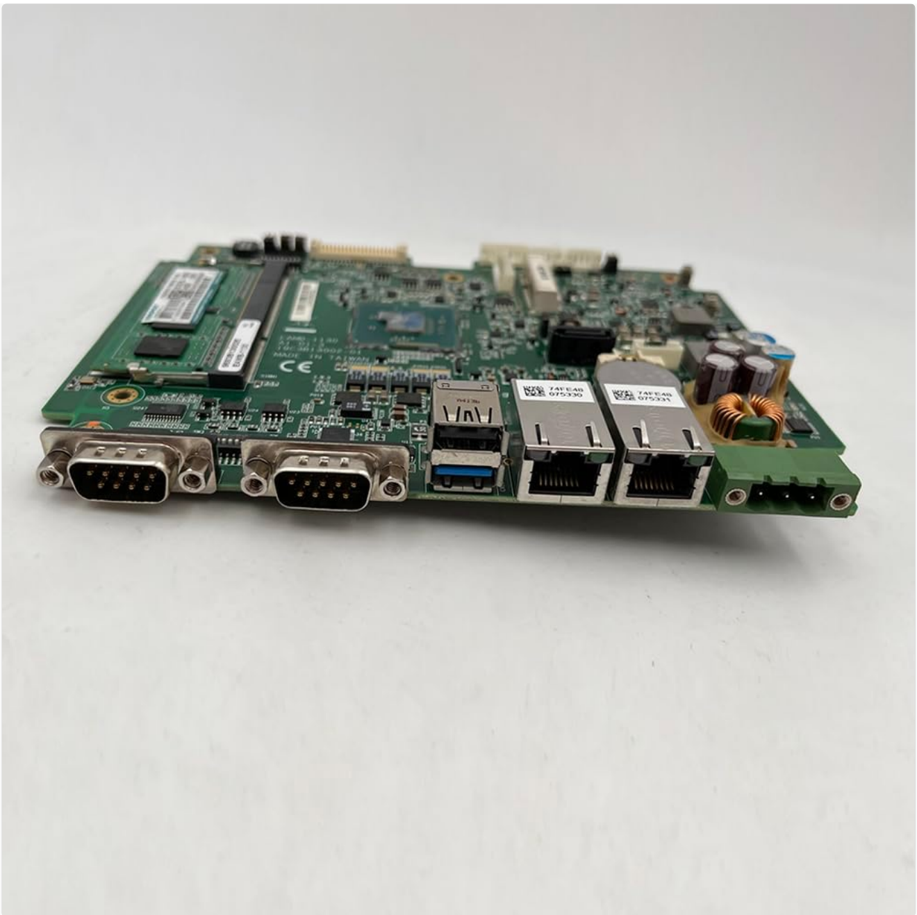
Figure 2.2: Side view of the EAMB-1130 motherboard. This image highlights the various input/output ports available on the board, including network and serial connectors.
