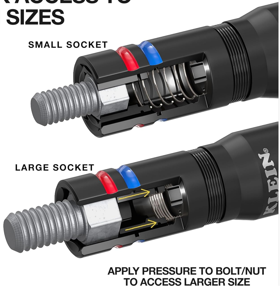
Image 3.1: Illustration demonstrating the spring-loaded mechanism for quick access to both small and large hex sizes within a single quad socket.
