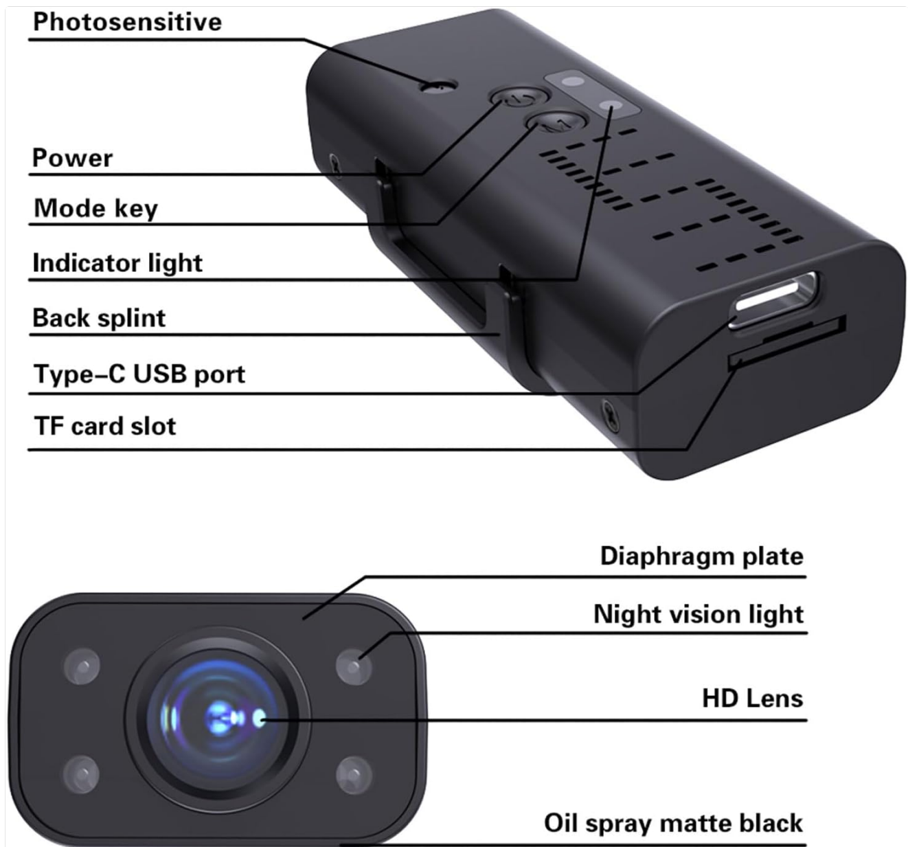
Figure 4.1: Labeled components of the Bewinner Wireless WiFi Camera.
