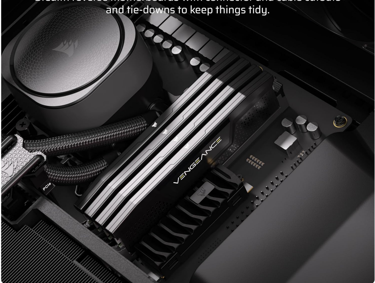
Figure 2.2: Close-up view of a motherboard designed for reverse connection, illustrating how the CORSAIR 5000D RS ARGB case accommodates such designs for improved cable routing.
