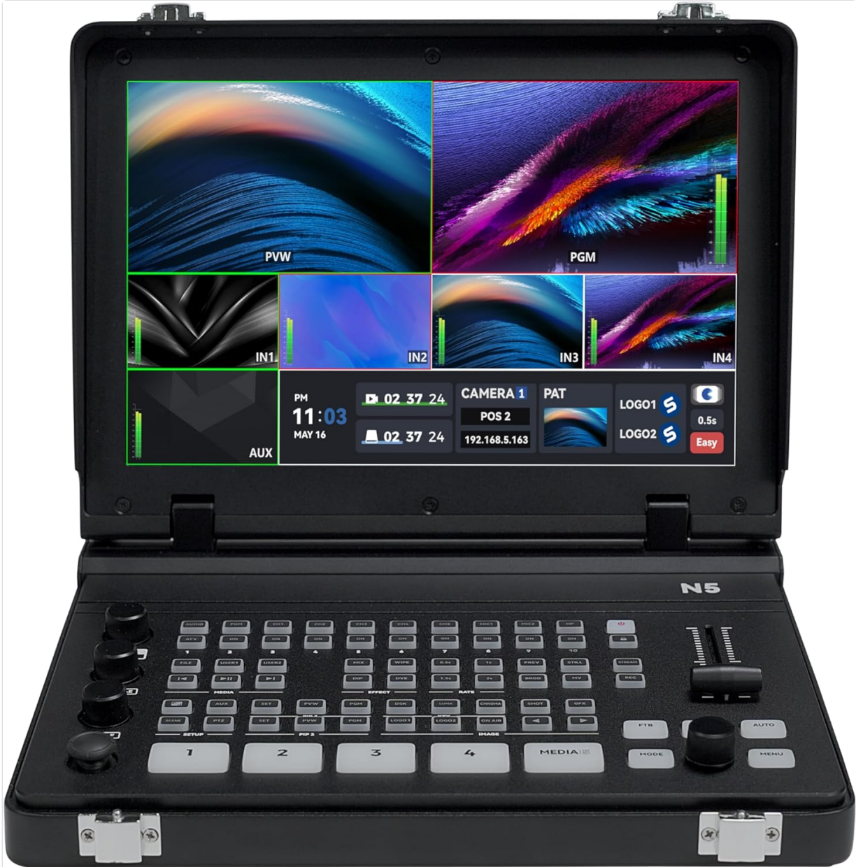
Image: Front view of the SPROLINK NeoLIVE N5, showing the integrated 10.1-inch display and the control panel with various buttons, knobs, and a T-bar for transitions.
