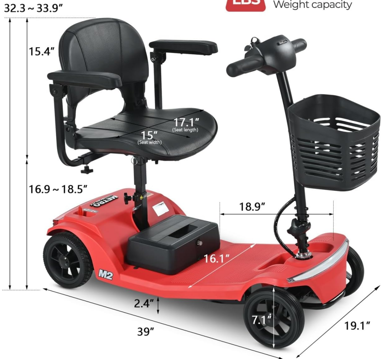
Figure 3.4: Overview of adjustable features including armrests, tiller, and seat height, along with the wider footrest and anti-tipping wheels.
