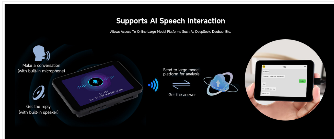
Figure 8: AI Speech Interaction. This diagram demonstrates the process of AI speech interaction, where the device captures voice input, sends it to an online large model platform for analysis, and receives a spoken or displayed response.
