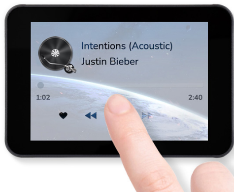
Figure 6: IPS Display and Capacitive Touch. This image demonstrates the excellent display performance with a 178-degree wide viewing angle and the responsive capacitive touch interface, suitable for human-machine interaction.
