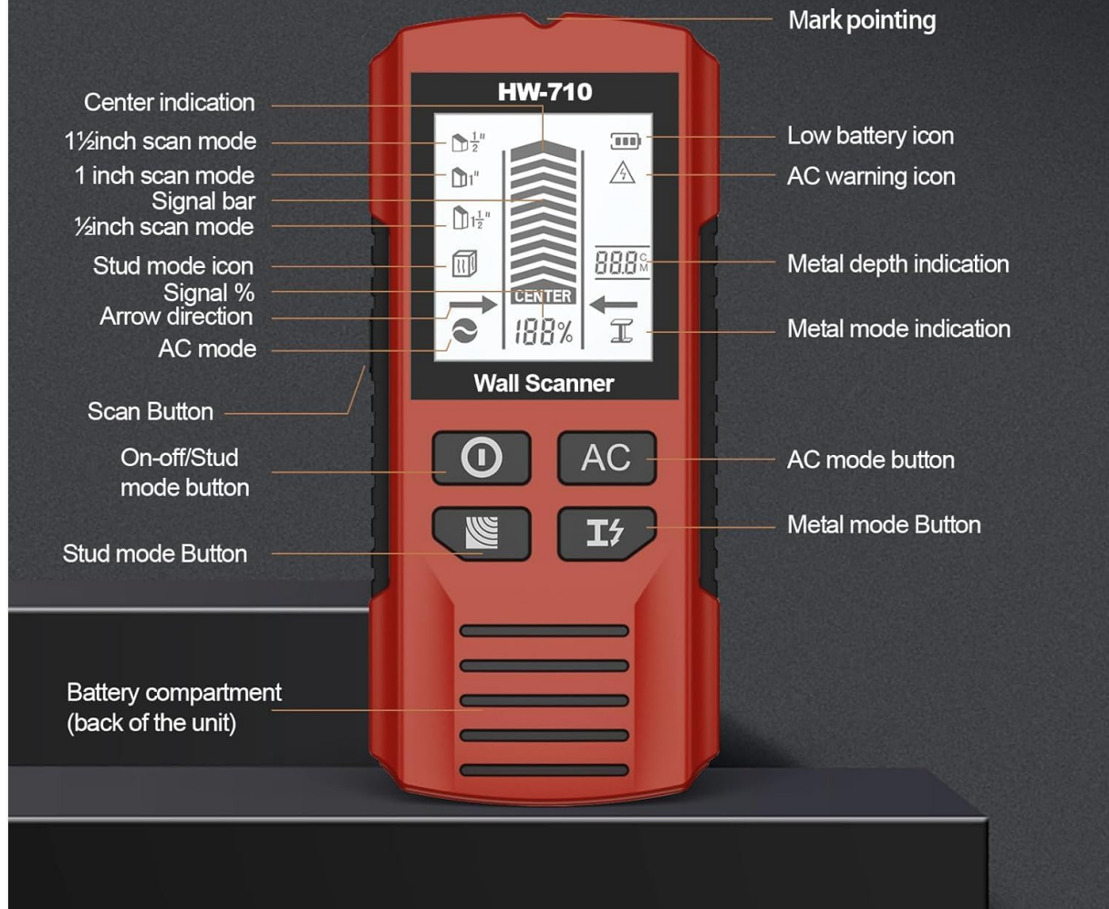
Image: Detailed diagram illustrating the functions of the HW-710's display and buttons, including scan modes, indicators, and battery compartment location.
