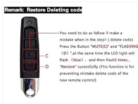
Image: Visual guide for clearing the cloning remote's memory, showing which buttons to press and the expected LED behavior.
