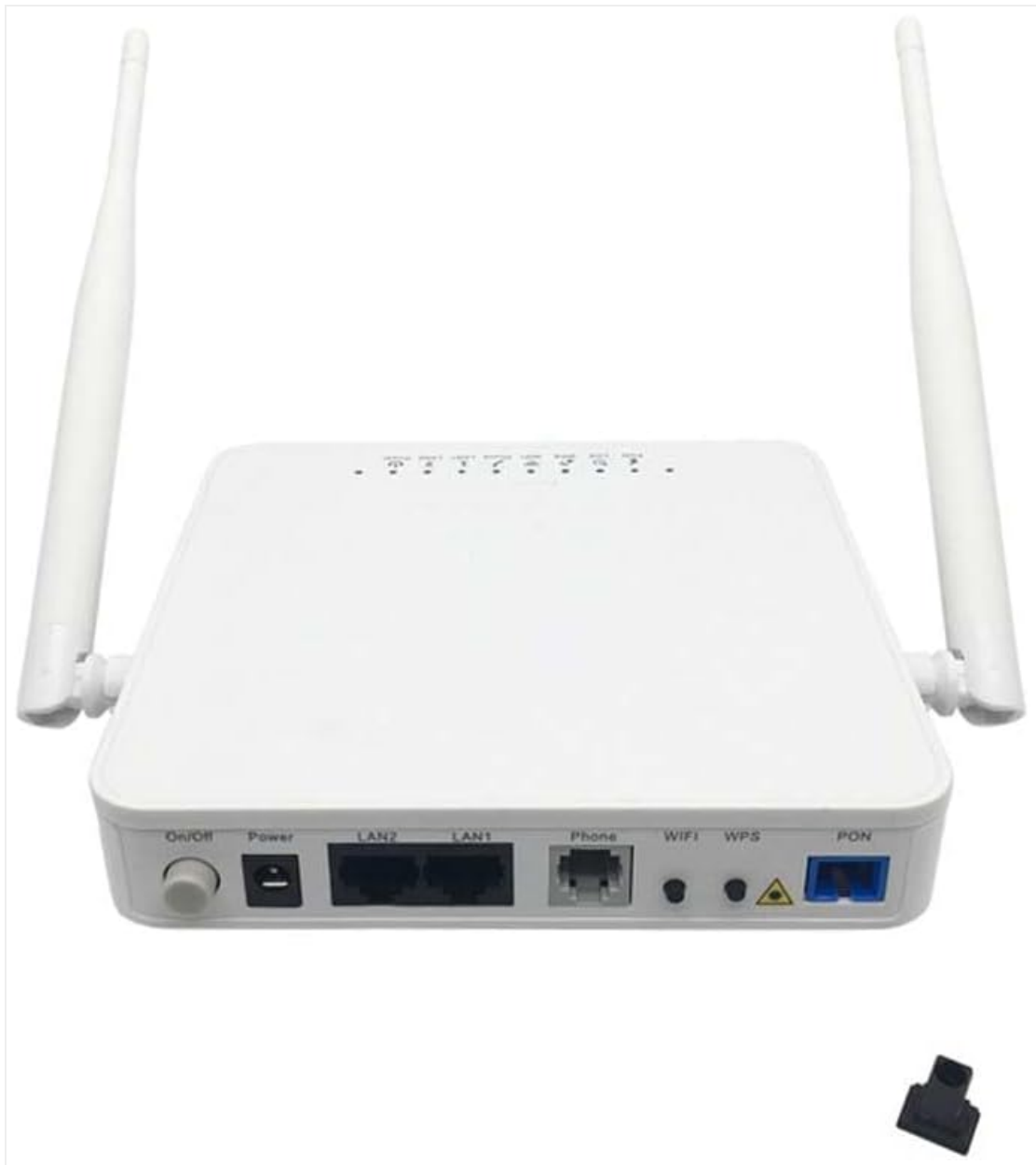
Figure 2.2: Rear View of the AN5506-02-FG. This image displays the back panel of the device, highlighting its various ports. From left to right, it features an On/Off button, a Power input, two LAN ports (LAN1, LAN2), a Phone port, a Wi-Fi button, a WPS button, and a PON optical fiber port. Two external antennas are also visible on either side.
