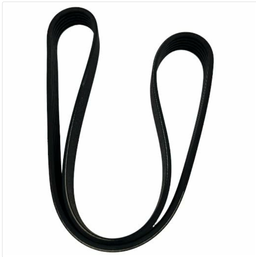
Image 4.1: A top view of the serpentine belt, illustrating its continuous loop design and the ribbed surface that engages with engine pulleys.
