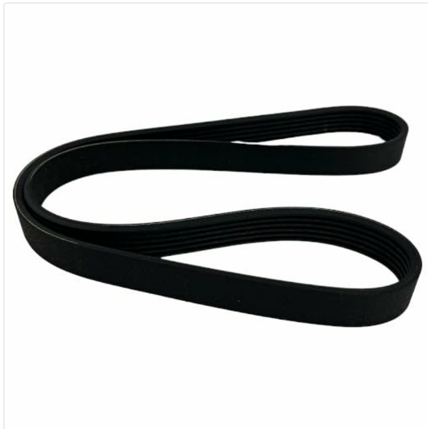
Image 3.1: A side view of the serpentine belt, showing the multiple ribs designed for efficient power transfer across various engine accessories.
