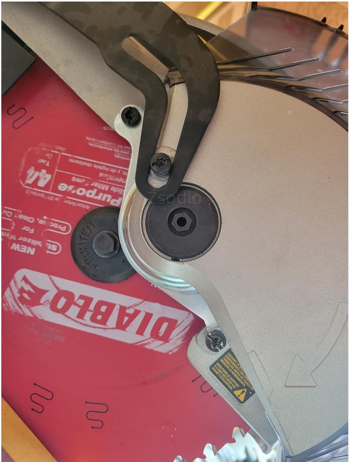
Figure 3: Zsodio 394589-01 screw installed in a Dewalt miter saw. This image shows the screw in its operational context, installed within a Dewalt miter saw. It demonstrates how the screw helps secure components, ensuring proper function and stability of the saw's rotating plate.
