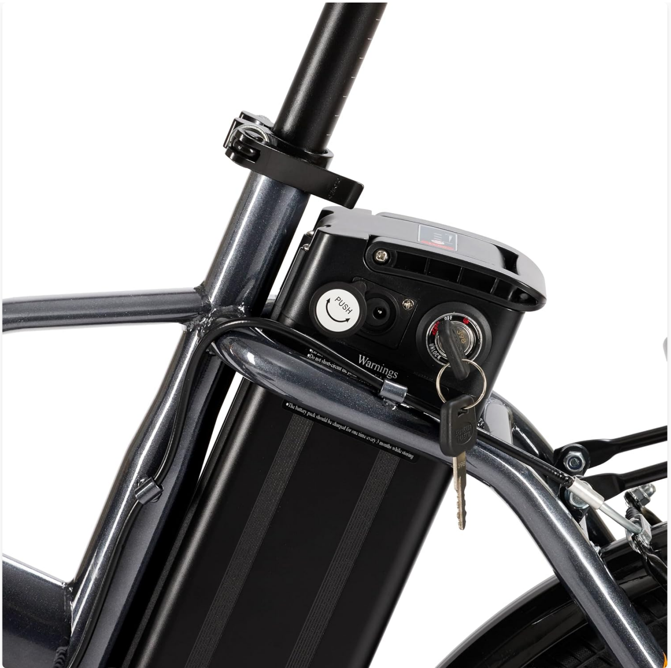
Image: Detail of the removable battery pack with key access.
