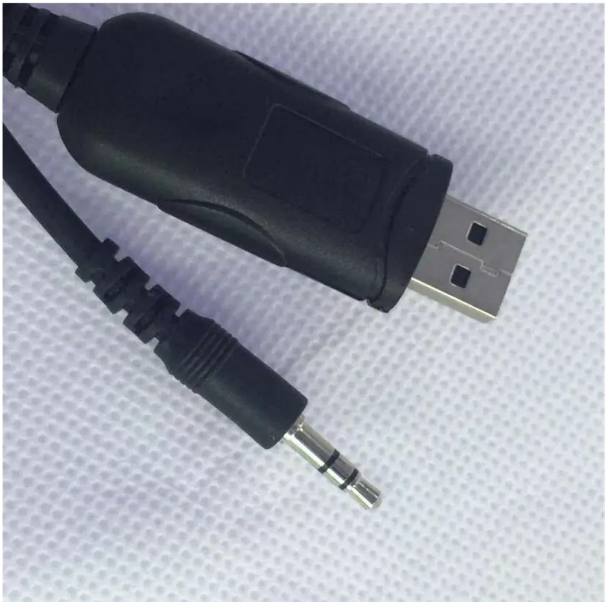
Figure 3: A close-up view showing both the USB-A connector and the 3.5mm audio jack of the programming cable, illustrating the
