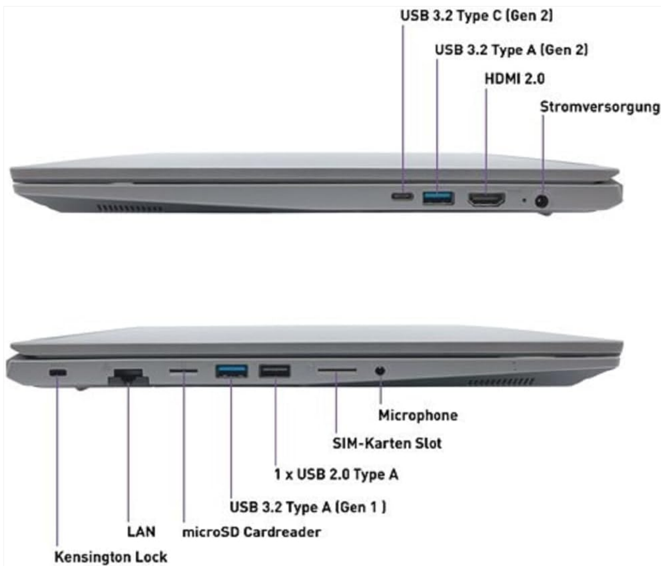
Figure 4.3: Detailed diagram illustrating the port configuration on the left and right sides of the laptop.
