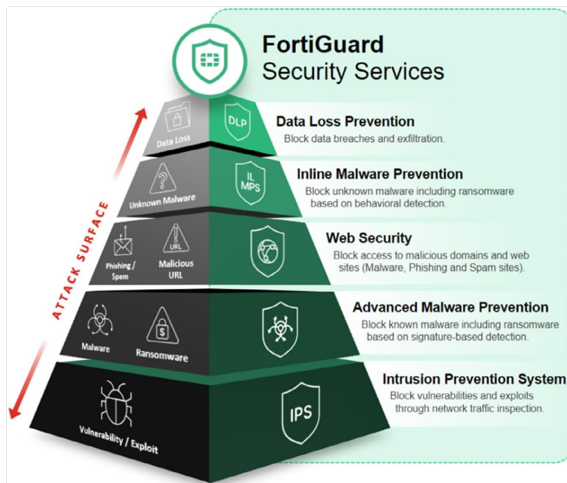
Figure 4.3: A pyramid diagram illustrating FortiGuard Security Services and their role in protecting against various attack surface elements, from Intrusion Prevention System (IPS) at the base to Data Loss Prevention (DLP) at the top.
