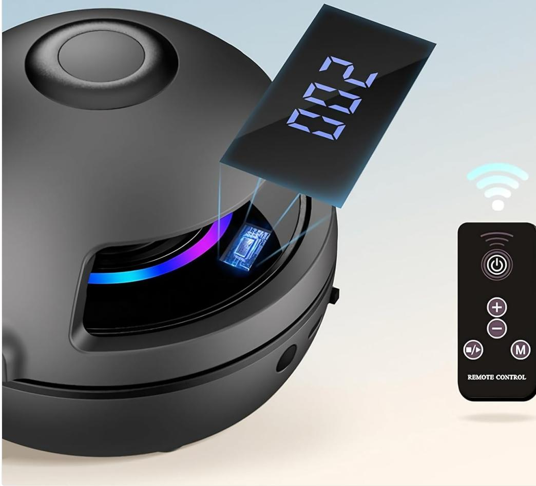
A detailed view of the machine's large LED display, which clearly shows the jump count and other relevant data, visible day and night.
