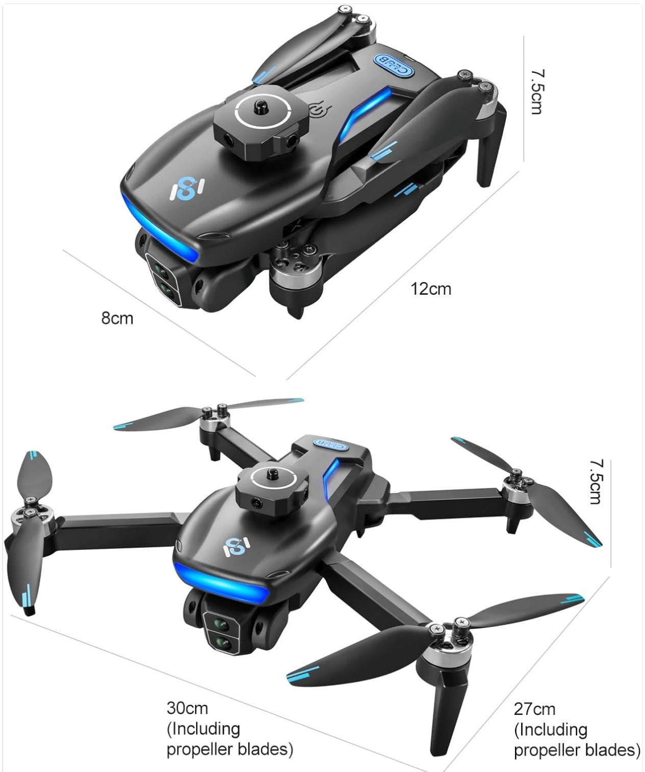
Figure 2.2: The drone shown in both its folded and unfolded configurations, highlighting its compact size and extended dimensions.
