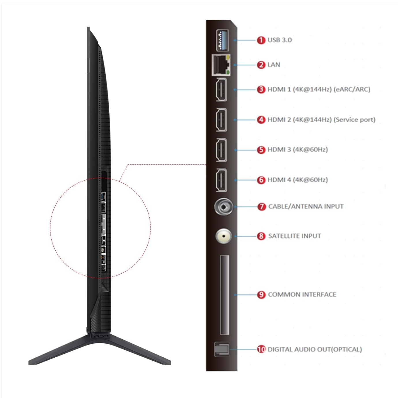
Detailed diagram of the TCL 55Q6C TV's side ports: 1. USB 3.0, 2. LAN, 3. HDMI 1 (4K@144Hz, eARC/ARC), 4. HDMI 2 (4K@144Hz, Service port), 5. HDMI 3 (4K@60Hz), 6. HDMI 4 (4K@60Hz), 7. Cable/Antenna Input, 8. Satellite Input, 9. Common Interface, 10. Digital Audio Out (Optical).
