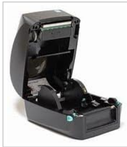
Figure 4.3: Internal view of the Godex RT730i+ printer with the top cover open, revealing the media loading area. This shows the path for labels and the ribbon mechanism for thermal transfer printing.
