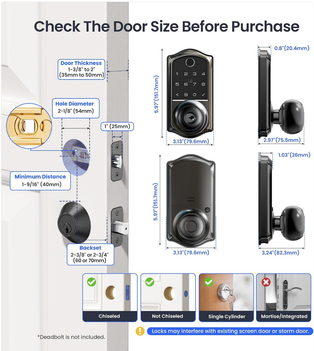
Image 2.1: Diagram illustrating required door dimensions (thickness, hole diameter, minimum distance, backset) for proper installation of the Veise VE018 Smart Lock. It also shows compatibility with chiseled and not chiseled doors, single cylinder, and incompatibility with mortise/integrated locks.
