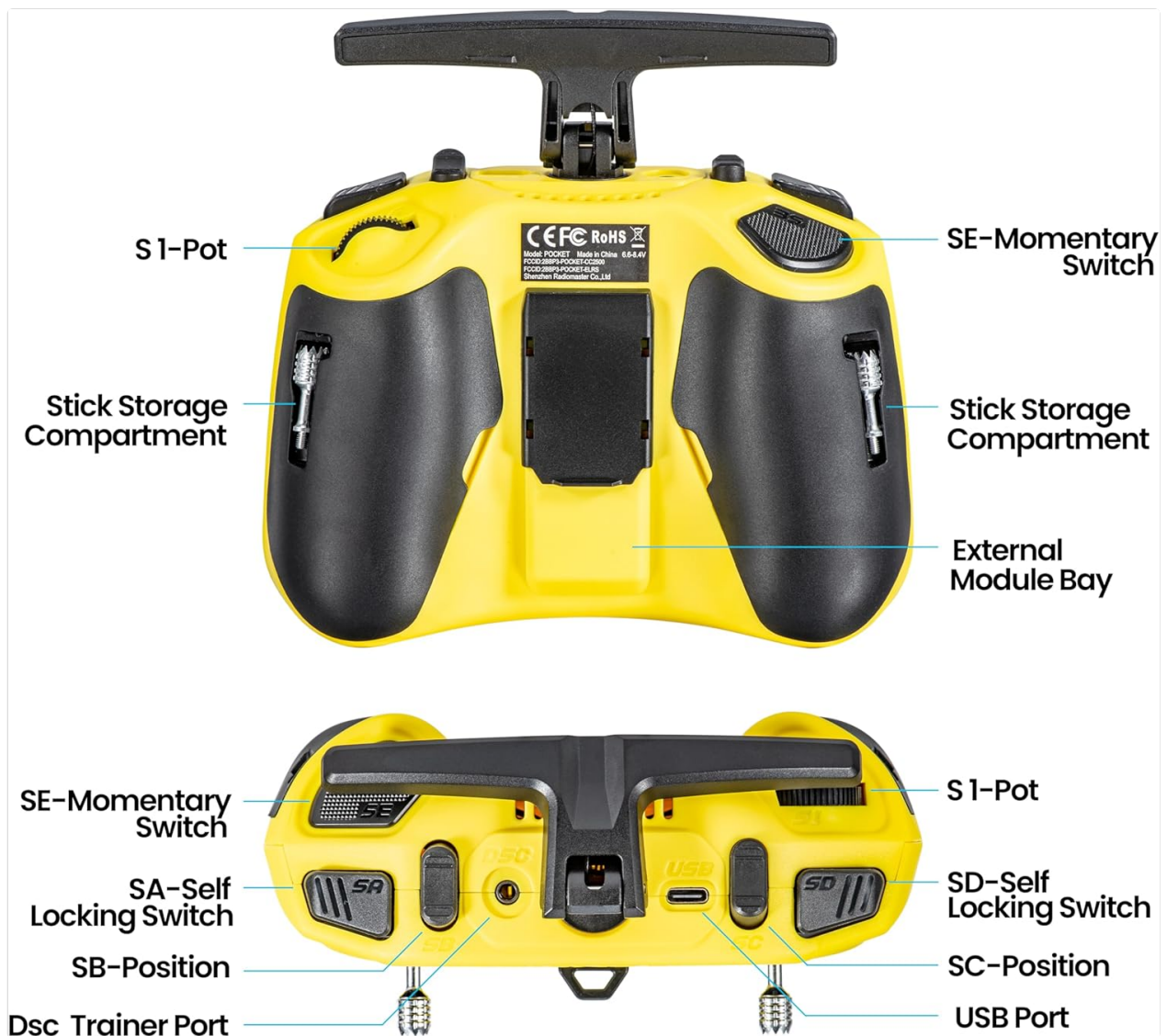
Image: Back and bottom view of the Radiomaster Pocket ELRS Remote Controller with labels indicating the S1-Pot, SE-Momentary Switch, Stick Storage Compartment, External Module Bay, SA-Self Locking Switch, SB-Position, SC-Position, SD-Self Locking Switch, DSC Trainer Port, USB Port, 3.5mm Headphone Jack, Type-C Charge Port, and SD Card Slot.
