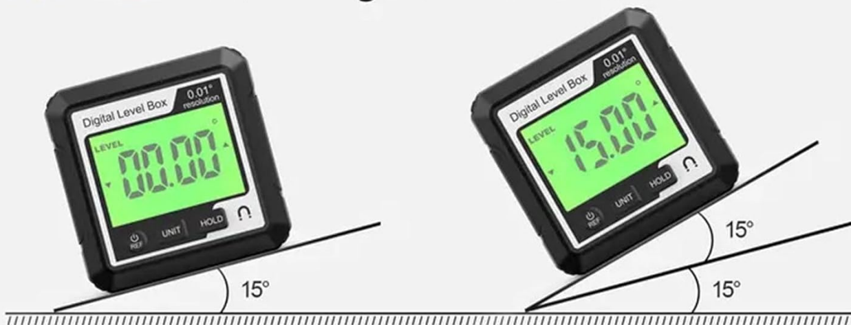
Figure 3: Illustration of Absolute Angle Measurement (Mode 1) and Relative Angle Measurement (Mode 2).
