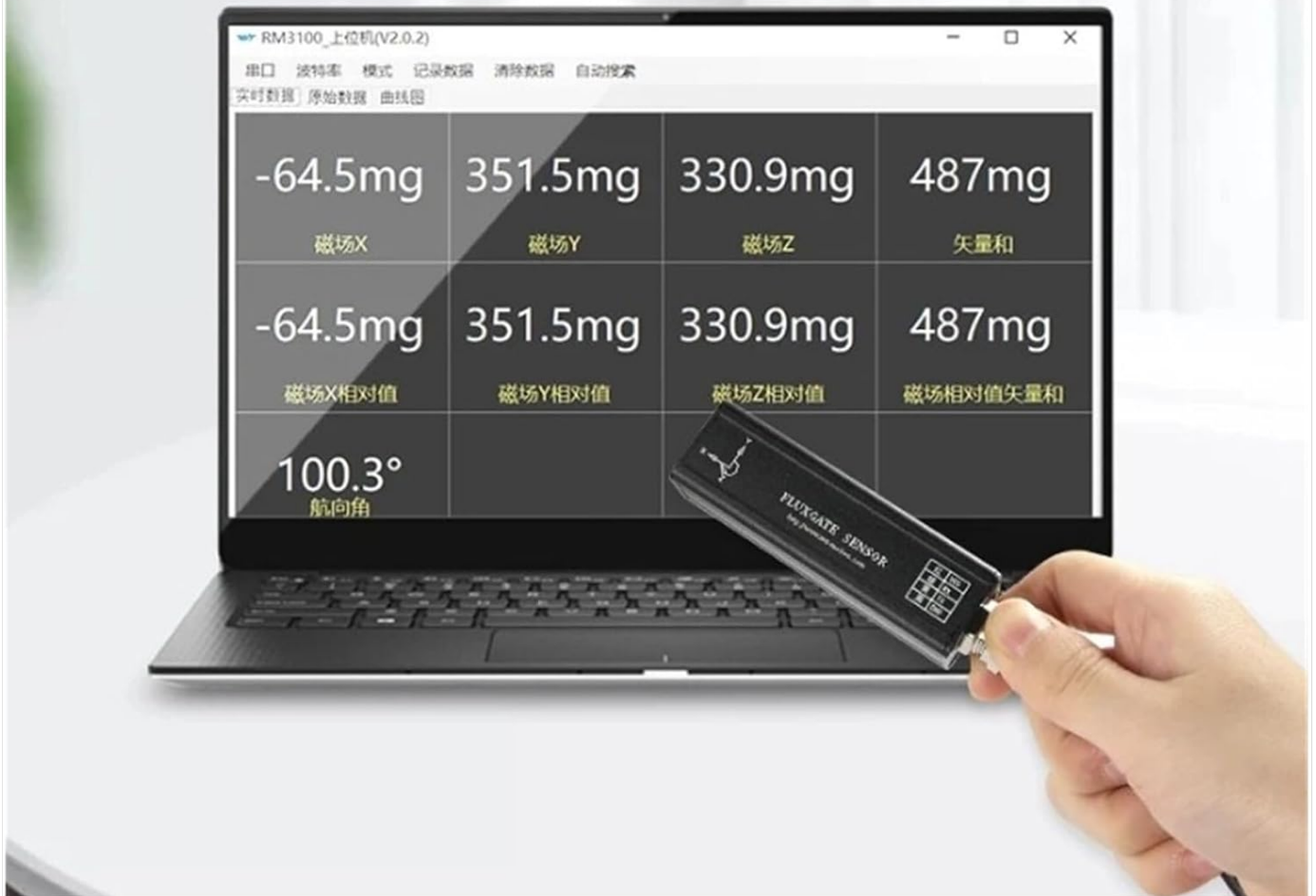
Image 3: Screenshot of a software interface displaying high-precision three-axis magnetic field output and heading angle. The image illustrates how the sensor's data can be visualized and processed.
