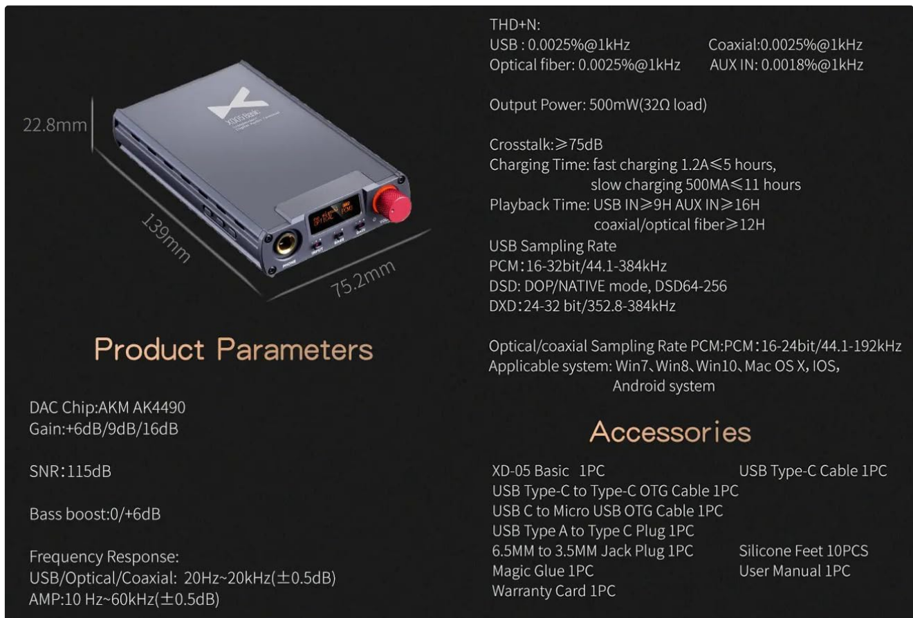
Figure 7: Detailed product dimensions and technical specifications. This image provides a visual representation of the device's size and a comprehensive list of its performance parameters.
