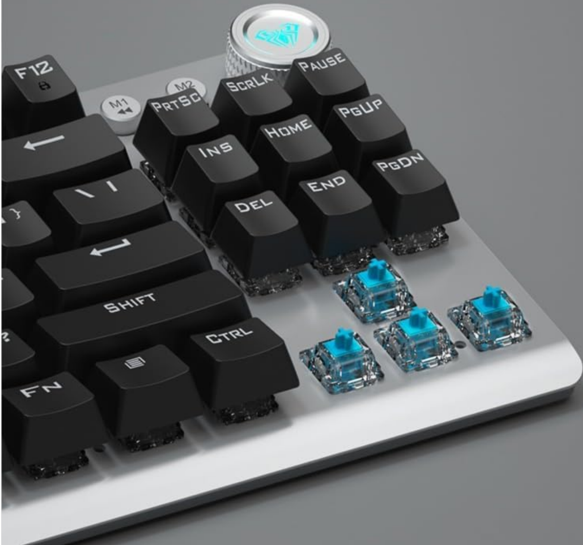
Figure 2: Detail of the keyboard's mechanical switches and the USB-C port for charging and wired connection.
