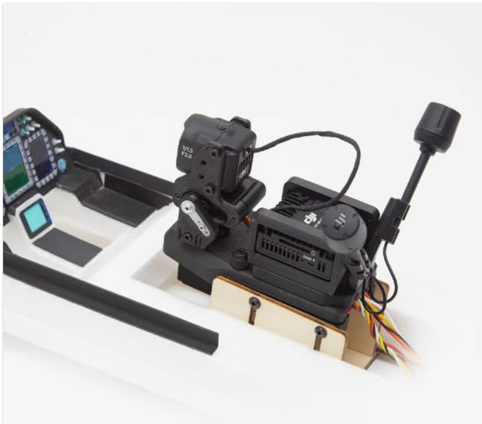
Figure 4.1: The ATOMRC Quick-Release Servo Gimbal V2 integrated into an FPV aircraft's cockpit, showcasing its compact design and wiring connections.
