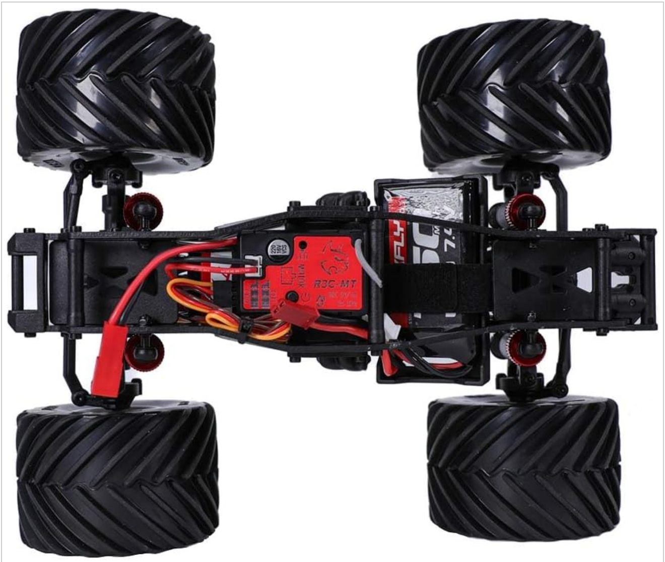
Image: An underside view of the Redcat Racing MT-18, highlighting the low CG 2mm aluminum chassis rails, metal drive shafts, and gear differentials.
