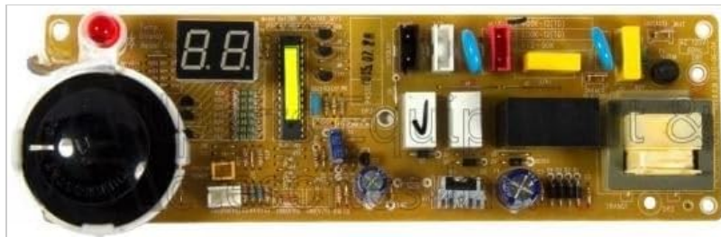
Figure 1: Top-down view of the Sourcefy 215A-0075-00 PCB Assembly, showing various electronic components, a digital display, and a control knob.
