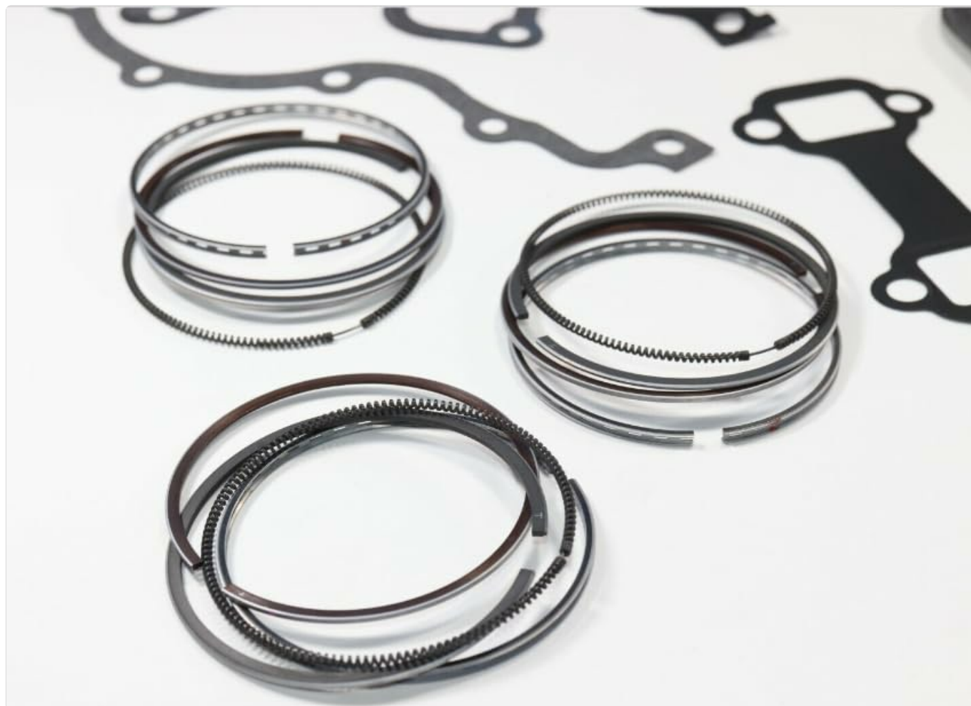
Figure 3.3: Detailed view of the three piston ring sets, essential for sealing the combustion chamber and controlling oil consumption.
