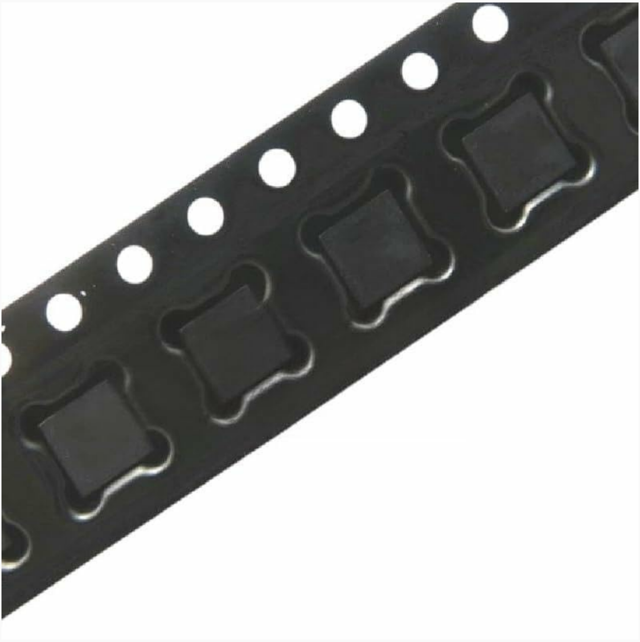
Figure 1: RT6807A/RT6807AZQV electronic components in tape-and-reel packaging. This image shows multiple small, square-shaped integrated circuits (ICs) embedded within a black plastic tape, with circular perforations along one edge for automated feeding during manufacturing.
