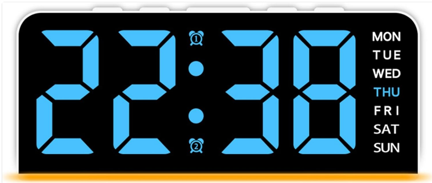
Figure 1: Front Display - Shows the large LED digits for time, and indicators for alarms and day of the week.
